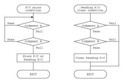
Note: 1): When Judgment A has failed, if Judgment B fails, SS C stuck off is detected. (See the diagram below)
