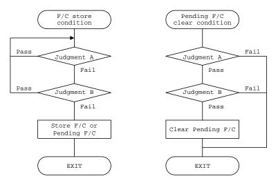
Note: 1): When Judgment A has failed, if Judgment B fails, SS C stuck on is detected. (See the diagram below)
